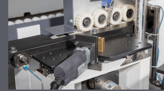
Servo Kontrollü Ön Siper Servo Controlled Entrance Fence
