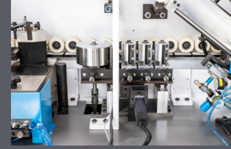
Servo Kontrollü Baskı Merdaneleri Pressure Rollers with Servo Control
