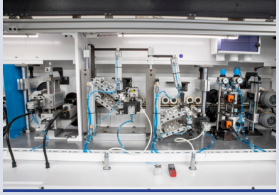
Servo Kontrollü Rounder Ünitesi Rounder Unit With Servo Control
