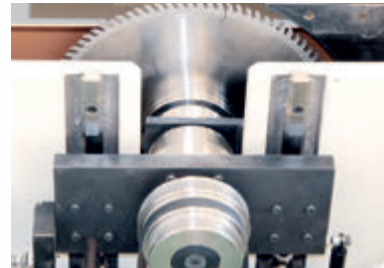
Linear Yataklı Ana Testere Ünite Hareketi Main Saw Blade Units Movement via Linear Guide
